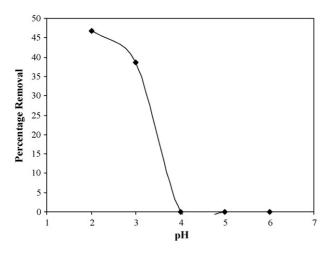
Fig. 1. Effect of pH on uptake of Tartrazine by hen feathers: temperature =  $50 \degree C$ ; concentration =  $9 \times 10^{-5}$  M; amount = 0.01 g; time = 24 h.
