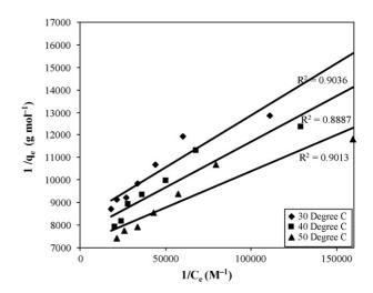
Fig. 4. Langmuir adsorption isotherm for Tartrazine–hen feather system: temperature  $= 50 \degree$ C; pH 2.0; amount = 0.01 g; time = 24 h.
