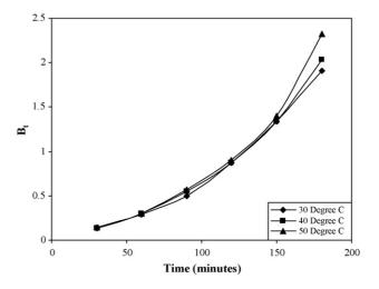
Fig. 8. Plot of time vs.  $B_t$  for Tartrazine uptake by hen feathers at different temperatures.
