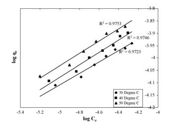
Fig. 3. Freundlich adsorption isotherm for Tartrazine–hen feather system: temperature = 50 °C; pH 2.0; amount = 0.01 g; time = 24 h.
