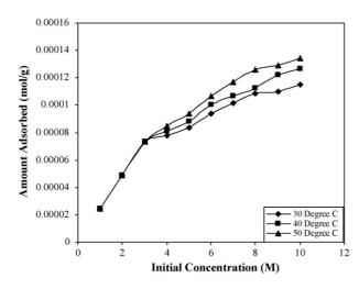
Fig. 2. Effect of concentration for the uptake of Tartrazine on hen feathers at different temperatures: temperature =  $50 \,^{\circ}$ C; pH 2.0; amount = 0.01 g; time = 24 h.
