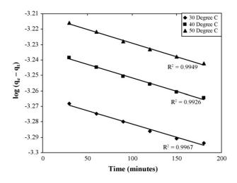
Fig. 7. Lagergren's plot of time vs.  $log(q_e - q_l)$  for Tartrazine adsorption on hen feathers at different temperatures.
