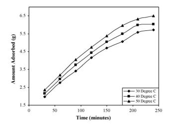
Fig. 5. Effect of contact time for the adsorption of Tartrazine by hen feathers at different temperatures: temperature =  $50 \degree C$ ; concentration =  $9 \times 10^{-5}$  M; amount = 0.01 g; pH 2.0.
