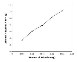
Fig. 6. Effect of amount of adsorbent for the removal of Tartrazine using hen feathers: temperature = 50 °C; concentration =  $9 \times 10^{-5}$  M; pH 2.0; time = 24 h.
